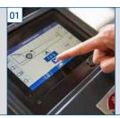
The new capacitive 7" touchscreen makes it particularly user-friendly and efficient to operate.
